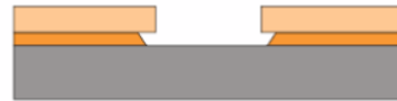
4. Develop resist and LOR. LOR develops isotropically, creating a bi-layer reentrant sidewall profile
